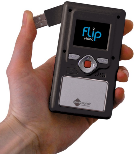
The FLIP camera fits in the palm of the hand, and downloads via USB thus making nearly instant video for posting. While its quality isn't professional, it is more than good enough for YouTube. In the new media world one shouldn't over emphasize video quality: Content, instead, is king!
